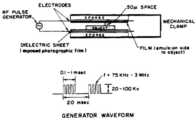
FIG. 2. Simple Kirlian photographic equipment and waveform using capacitor-plate configuration.
