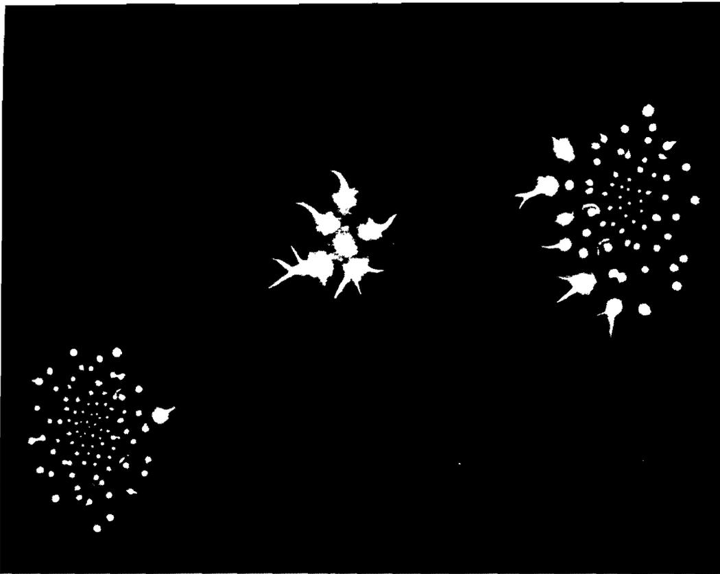
FIG. 7. Photograph of fingertip for different spacing between finger at electrode-film surface. Pulse width = 100  $\mu$ sec, single pulse. Discharge space  $d$  is largest for center photo (3 $\times$ ).
