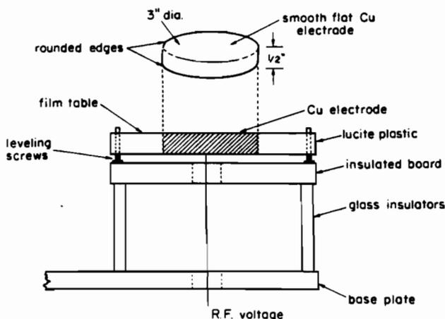
FIG. 5. Single-electrode configuration for photographing fingertips.
