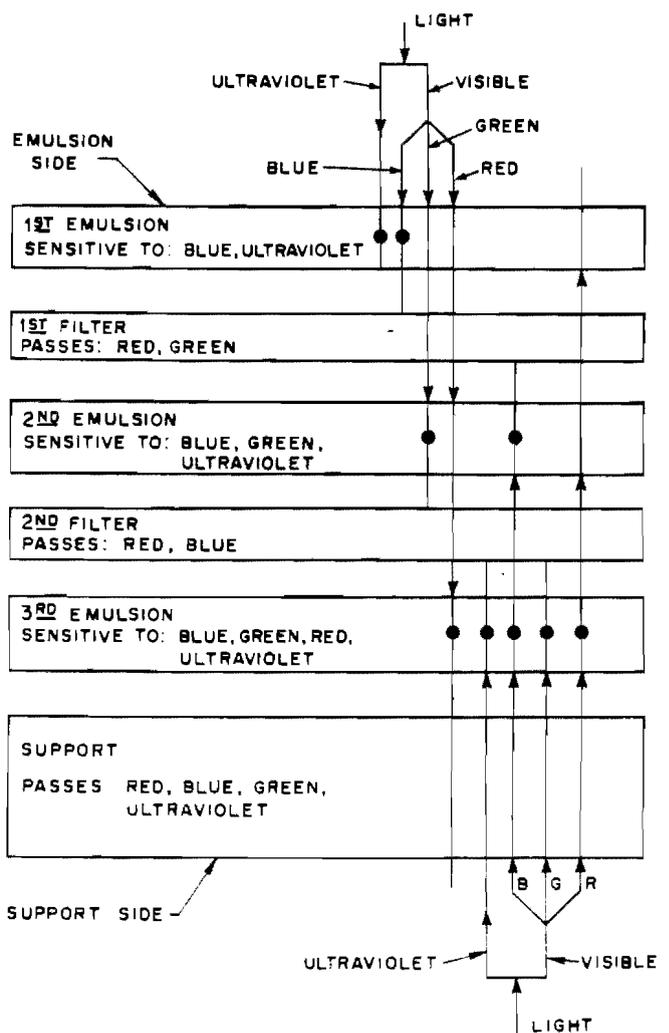
FIG. 13. Color film construction, a schematic representation of the effect of uv and visible light exposing the film from the emulsion side vs from the support side. Dot in light path indicates exposure of emulsion. (Note that the film actually uses a subtractive color system of yellow, magenta, and cyan. See Ref. 11.)
