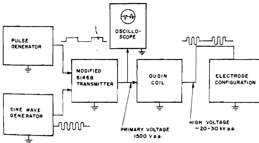
FIG. 3. Block diagram of equipment built by authors.
