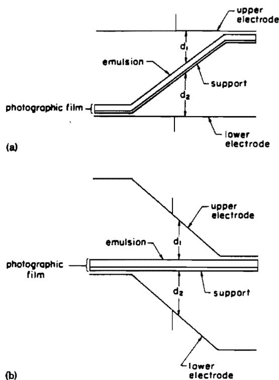
FIG. 14. Representation of film bending shown in exaggerated scale. (a) Film bent, electrodes planar; film exposure from left to right will be blue, white (blue, red, green), and orange (red, green), respectively. (b) Equivalent topological configuration to that in (a), except the electrodes are bent and the film is planar. All intermediate combinations at (a) and (b) are possible.
