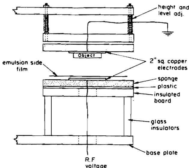
FIG. 4. Initial electrode configuration mounted on an alignment device.
