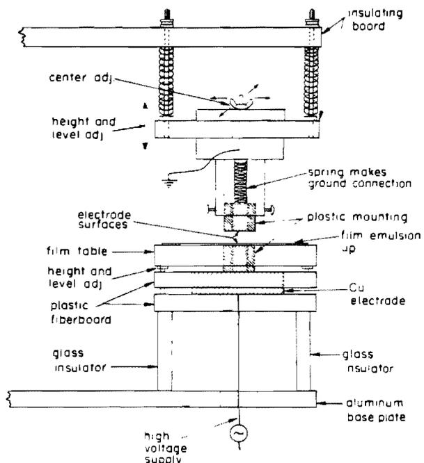
FIG. 8. Electrode holder for polished metal electrodes. Electrodes are fixed in a plastic mounting and placed in a parallel configuration in the apparatus, as shown.
