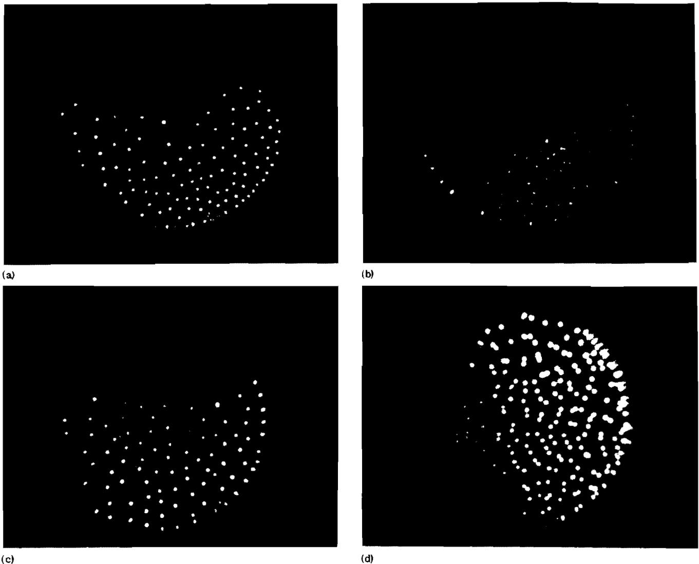
FIG. 10. Photographs of discharge between flat polished stainless-steel electrodes under conditions of different pulse exposure, electrode spacing, and orientation ( $3.7\times$ ). (a) Pulse width =  $400\ \mu\text{sec}$  and single pulse. (b) Pulse width =  $200\ \mu\text{sec}$ , rep. rate =  $1\ \text{Hz}$ , duration = 2 pulses. (c) Pulse width =  $500\ \mu\text{sec}$ , single pulse. (d) Pulse width =  $500\ \mu\text{sec}$ , rep. rate =  $1\ \text{Hz}$ , duration = 2 pulses.
