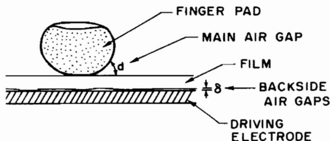
Fig. 6. Schematic illustration of discharge gap distance  $d$  for a fingerpad-film combination plus the small air gaps of distance  $\delta$  between the film and the back side of the electrode.
