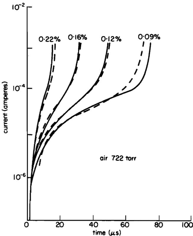
**Fig. 2.** Comparison of current,  $I$ , growth in air for various constant overvoltages obtained experimentally by (-----) by Bandel and calculated by Ward.
