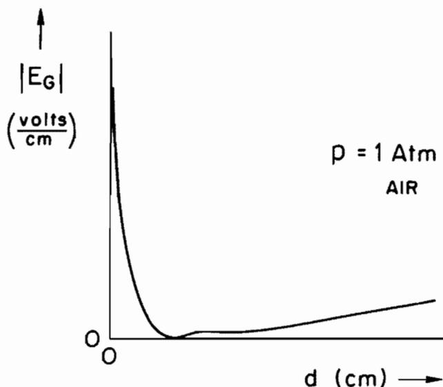
Fig. 5. Plot of absolute value of electric field strength  $|E_G|$ , for air in the gap as a function of electrode separation distance,  $d$ , for  $p = 1$  atmosphere.
