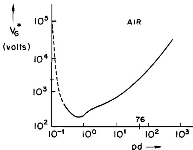
Fig. 1. Schematic illustration of air breakdown voltage,  $V_G^*$ , as a function of the product, gas pressure,  $p$  (in mms) X electrode spacing,  $d$  (in cms).
