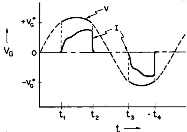
**Fig. 3.** The gap voltage,  $V_G$ , and discharge current,  $I$ , as a function of time for metallic electrodes (zero wall-charge case) indicating that significant current flows only when  $V_G$  exceeds the critical voltage  $V_G^*$ .
