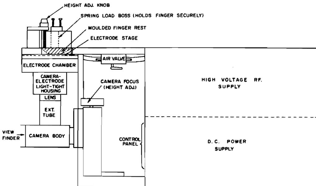
3. (a) Functional diagrams of the transparent electrode device.
