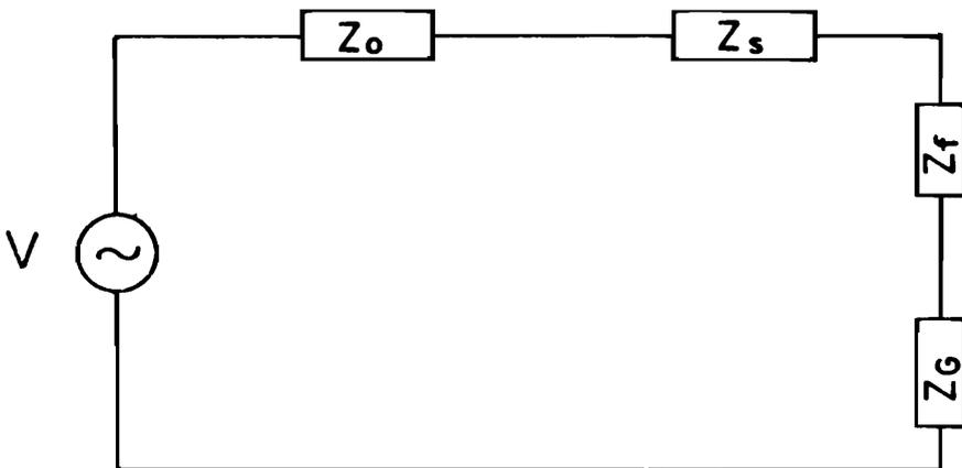
Fig. 4. Circuit elements in typical Kirlian photography system.
