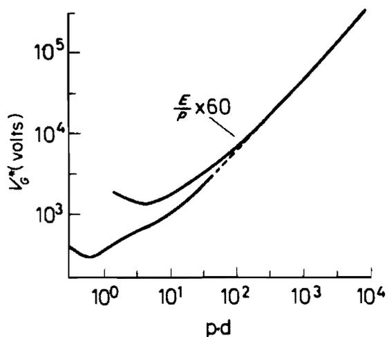
Fig. 5. Experimental (lower) and calculated (upper) curves showing the relationship between breakdown voltage,  $V_G^*$ , and  $p.d$  for air at 1 atm [9].
