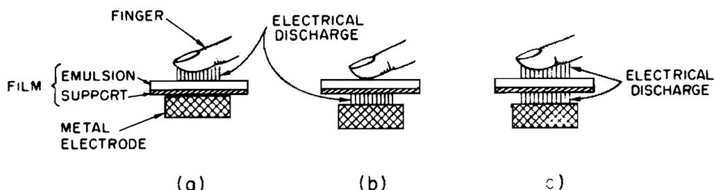
Fig. 2. Three modes of film exposure via light produced by the electrical discharge in air gaps between either/both film and finger and film and metal electrode (the actual discharge becomes normal to the finger surface).
