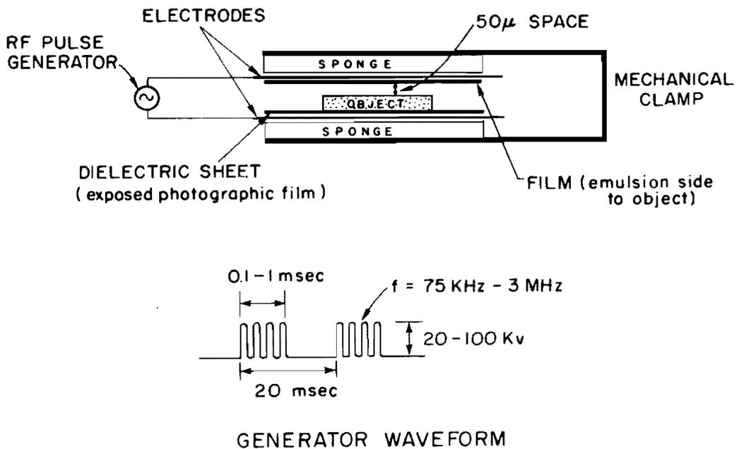
Fig. 1. Simple electrode device and power supply characteristics used in Soviet Kirlian photographs of leaves and other simple objects.
