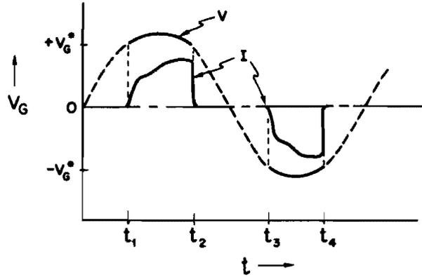
Fig. 7. The gap voltage,  $V_G$ , and discharge current,  $I$ , as a function of time indicating that significant current flows only when  $V_G$  exceeds the critical voltage  $V_G^*$ .
