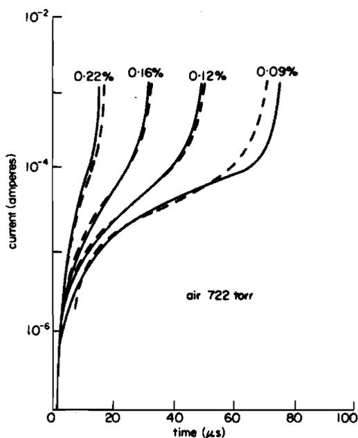
Fig. 6. Comparison of current growth with time in air for various overvoltages obtained experimentally [10] (dashed) and calculated [11] (solid).
